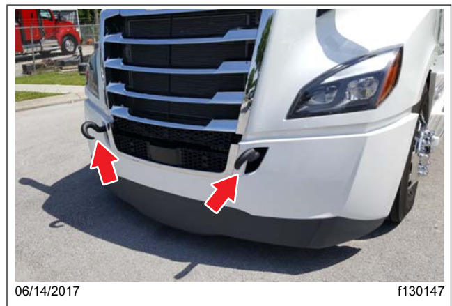
Fig. 23.7, Tow Hooks Installed, Facing Down
