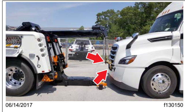
Fig. 23.9, Tow Cables Connected to the Tow Hooks
