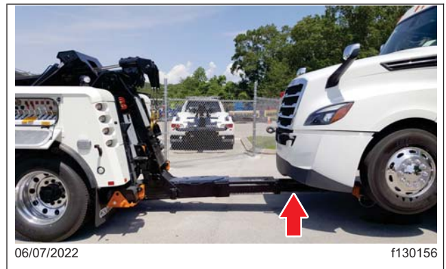
Fig. 23.15, Retracting the Recovery Boom
