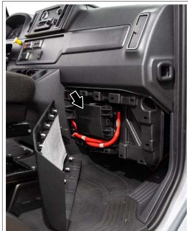
Fig. 8.7, Power Distribution Module (PDMi) Behind Right-Side Dash
