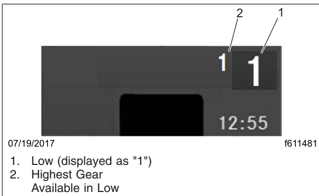
Fig. 14.14, Allison Gear Display in Low Gear
