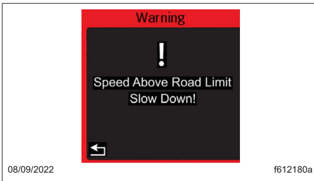
Fig. 6.26, Traffic Sign Display Warning
