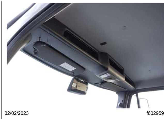
Fig. 3.46, Overhead Instrument Panel
